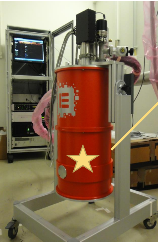
Adiabatic Demagnetization Refrigerator (ADR)
