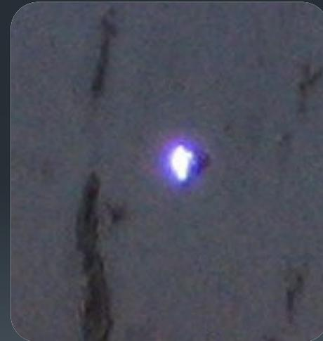
*A laser spark on Aluminium at 60 m distance*
