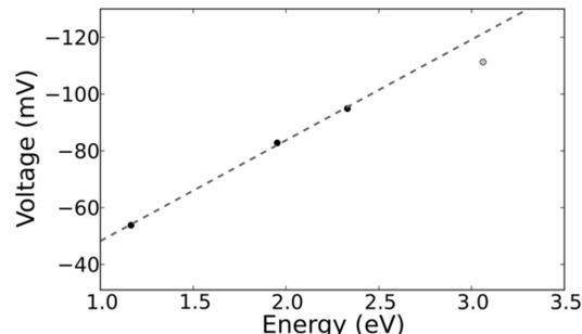
Average pulse height in units of voltage output as a function of photon energy for the TES. The dashed line is a fit to the first three points.
