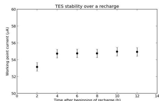
The TES working point current equivalent to  $RO = 30\%$   $R_{normal}$  as a function of time after the beginning of a recharge.
